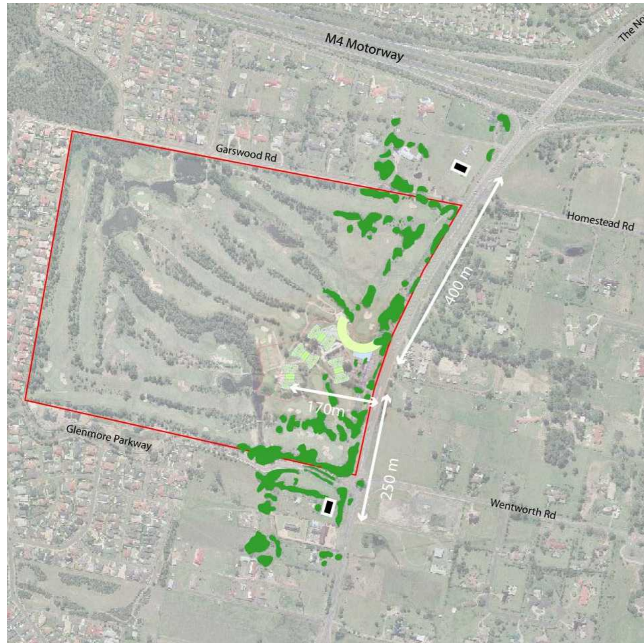
FIGURE 13: BUILDING SETBACKS + SEPARATION
